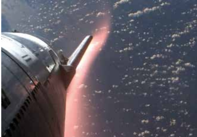
▲ A camera aboard the SpaceX Starship records the build-up of plasma as the vehicle re-enters the atmosphere at the end of its flight on 14 March 2024. [Credit: SpaceX]
